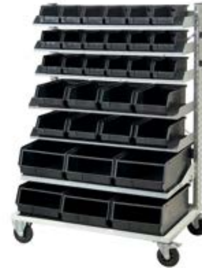
Item Code FLB B101 52 52 Dimensions in inches 40.28x24.13x56.30 H Full cart with: 1 cart Item FLB B101 02 52 18 18 ZEUS containers Mod. 2PLZ 8 ZEUS containers Mod. 3A2PLZ 6 ZEUS containers Mod. 4PLZ 2 swivel casters with brake Ø4.92 inches 2 rigid casters Ø4.92 standard rubber Load capacity 661.4 lb (330.69 lb each side)
