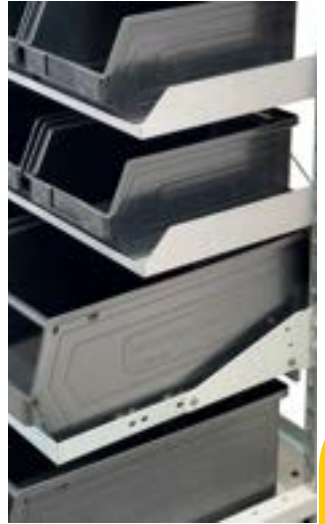
Item Code FLB B101 52 52 Dimensions in inches 40.28x24.13x56.30 H Full cart with: 1 cart Item FLB B101 02 52 18 18 ZEUS containers Mod. 2PLZ 8 ZEUS containers Mod. 3A2PLZ 6 ZEUS containers Mod. 4PLZ 2 swivel casters with brake Ø4.92 inches 2 rigid casters Ø4.92 standard rubber Load capacity 661.4 lb (330.69 lb each side)
